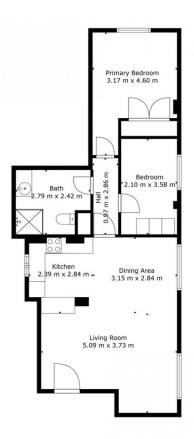
GROSS INTERNAL AREA FLOOR 1: 63 m2 TOTAL: 63 m2 Measurements Are Calculated By Cubicasa Technology. Deemed Highly Reliable But Not Guaranteed.
